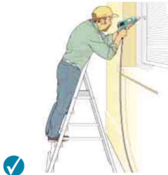
Figure 7b Correct - steps facing work activity
