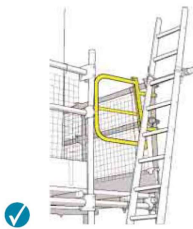
Figure 4 Access ladders tied and extending above the landing point
