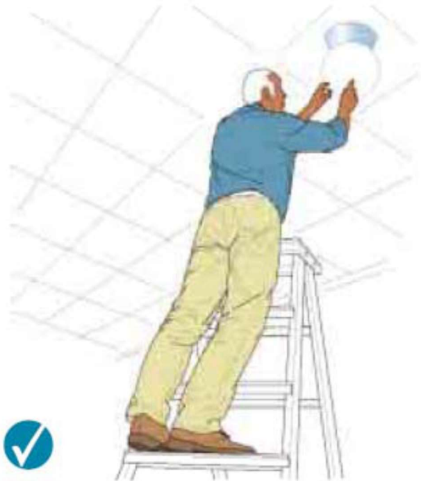
Figure 6b Correct - 3 clear rungs. Don't work any higher up this type of stepladder.
